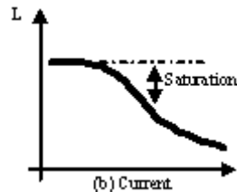
Figure 2b. Saturation effects of an SoC inductor with respect to current
