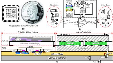
Figure 1. (a) A self-powered SOC with fully integrated micro-fuel cell hybrids, (b) its power scheme and management circuits, and (c) its physical profile view.
