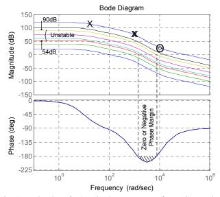
Fig. 1: Bode Plot of a 3-pole, 2-zero system for various values of low-frequency gain LG<sub>FB0</sub>.
