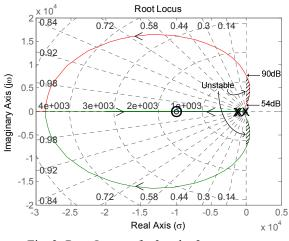
Fig. 2: Root Locus of a 3-pole, 2-zero system.
