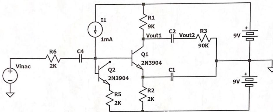
The collector of Q2 is left unconnected making Q2 function as a Diode and NOT a transistor (a diode connected transistor). Thus, Q2's BE junction can be treated as a diode for BOTH DC AND SMALL SIGNAL. Thus, you may want to replace Q2 with a Diode for clarity. 2N3904 Beta=100,  $V_a=300V$  and  $I_s=1e-14A$  with a  $V_{be}$  Turn On voltage of 0.66V
