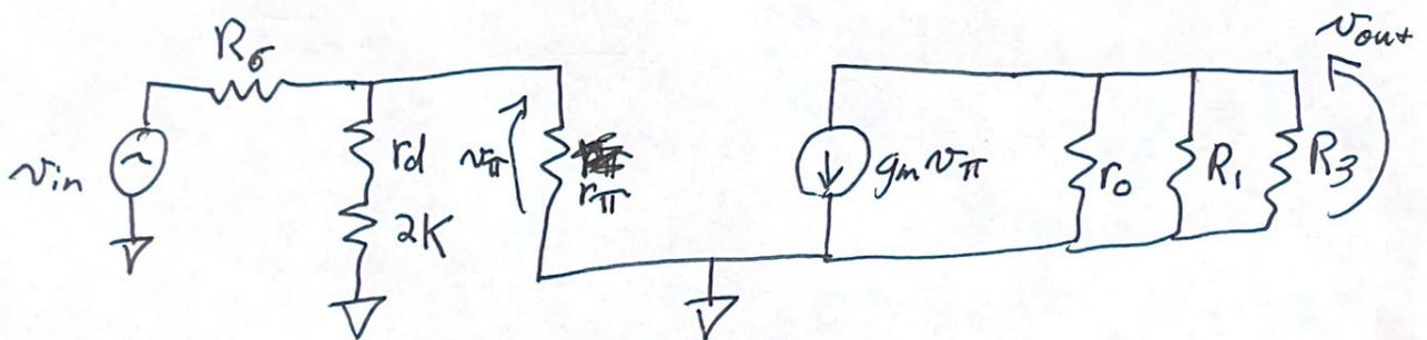
$$\left( \frac{v_{\pi}}{v_{in}} \right) = \frac{r_{\pi} \parallel (r_d + 2k)}{R_G + r_{\pi} \parallel (r_d + 2k)} = 0.362 \text{ V/V}$$
