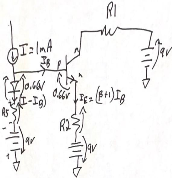
$$-9V + (I - I_B)R_5 + 0.66V - 0.66V - I_B(\beta + 1)R_2 + 9V = 0$$
