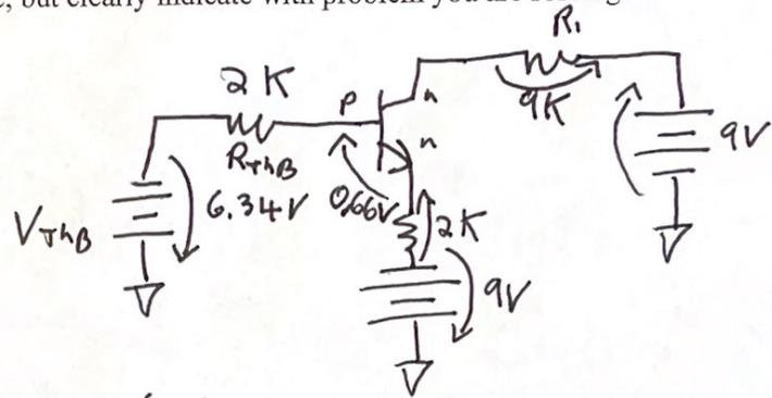
$$-6.34V + I_B(2k) - 0.66V - \underbrace{(1+\beta)I_B 2k}_{I_E} + 9V = 0$$
