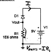
The diode is to be used as a photodetector biased with the circuit shown. Find the value of the output voltage, Vout, for (a. 10-points) dark conditions where there is no light and (b. 10-points) for lighted conditions when a generation rate of 1e19 electron-hole pairs/cm<sup>3</sup>-Second illuminates the diode.
