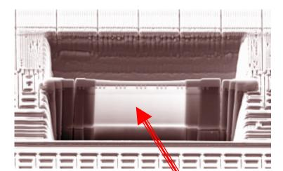
TEM lift-out sample after milling and polishing. Note the electron transparency of the thin area.
