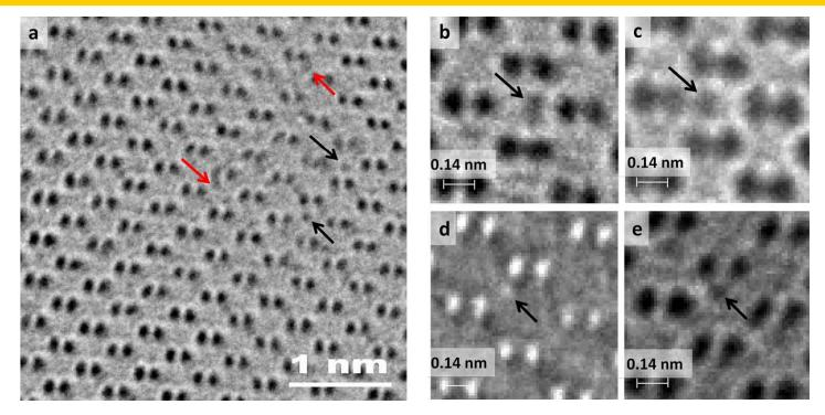
Aberration-corrected images of a thin Ge crystal; black arrows: occupied interstitial sites, red arrows: dark gray show column vibrations occurring during the acquisition time
