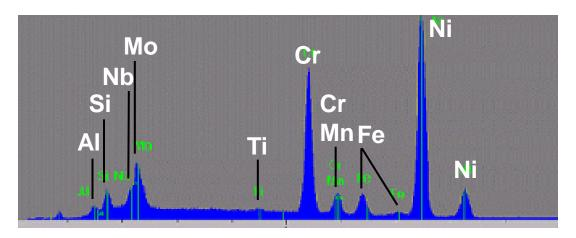
Nickel-based alloy consisting of *nickel*, *chromium*, *manganese*, *titanium*, *silicon*, *molybdenum*, and *aluminum*
