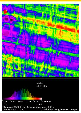
EBIC image (left) and EBIC-DLM image (right) showing non-uniform electrically active defects in a SiC epitaxial sample. Diffusion length varies by more than a factor of 4 in this sample. Non-uniformity is due to poor polishing of the SiC substrate and subsequent variation in the epitaxial film surface recombination velocity at the film-substrate interface.
