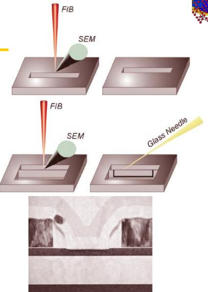
30-kV bright field STEM image of a semiconductor structure showing a small defect in the center.
