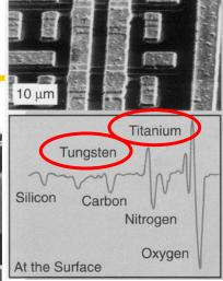
Residual TiW monolayer in PROM link was identified with scanning AES; responsible for charge leakage.
