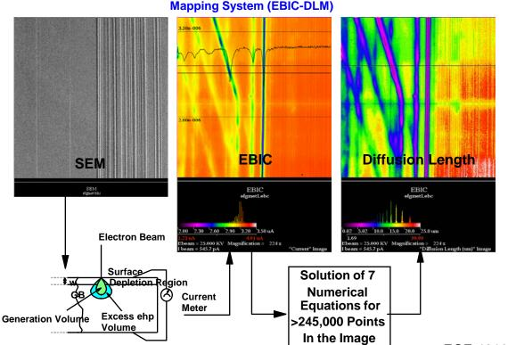
**Electron Beam Induced Current (EBIC) and EBIC Diffusion Length** Mapping System (EBIC-DLM)
