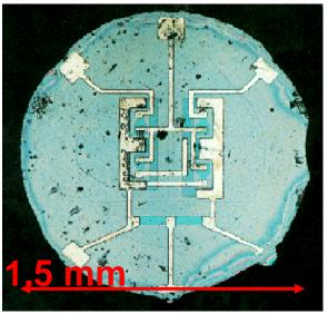
First Planar IC 1961, Fairchild http://smithsonianchips.si.edu/ IBM 200 mm and 300 mm wafer http://www-3.ibm.com/chips/photolibrary
