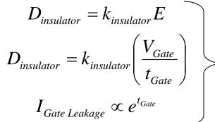
Gate leakage current can be dramatically lowered by increasing Gate insulator thickness but to do so without changing the channel conductivity, you have to increase the dielectric constant of the insulator. NEW GATE INSULATORS FOR THE FIRST TIME IN 60 YEARS!!!!
