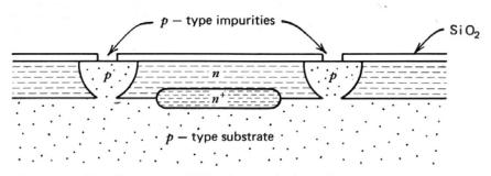
Figure 2.12 Structure following isolation diffusion.
