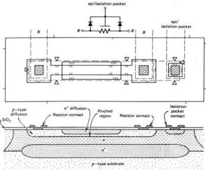
Figure 2.32 Pinch resistor structure
