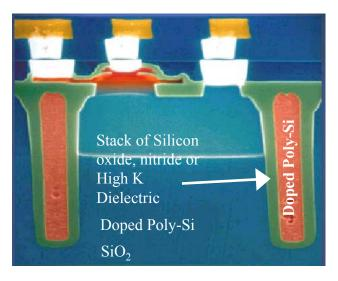
Figure 2.55b Plan view and cross section of typical poly-poly capacitor.
