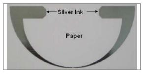
Figure 1. Silver based half-wavelength tapered-width U-shaped antenna
