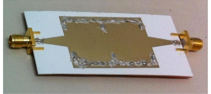
Figure 6. Photograph of the SIW filter on paper.
