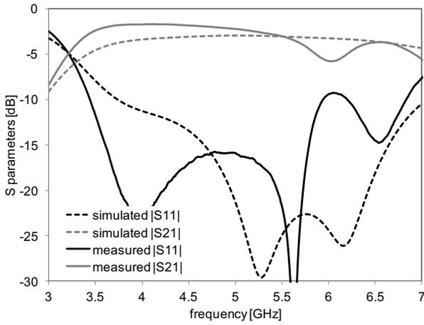
Figure 3. Simulated and measured scattering parameters of the SIW transmission line on paper.
