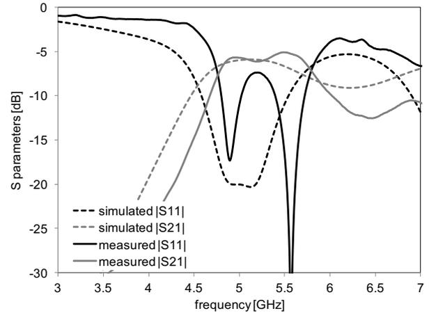
Figure 7. Simulated and measured scattering parameters of the SIW filter on paper.
