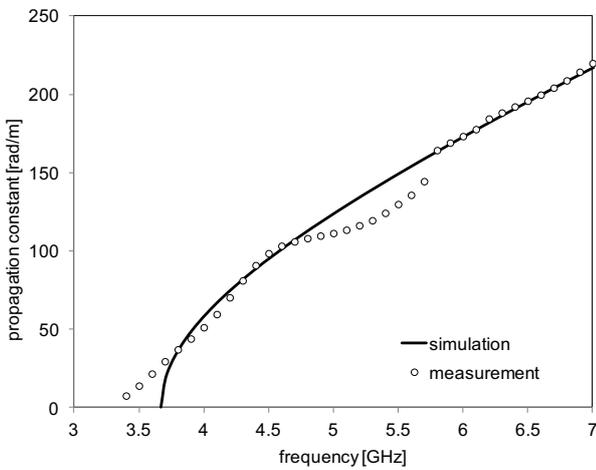
Figure 4. Simulated and measured propagation constant of the SIW transmission line on paper
