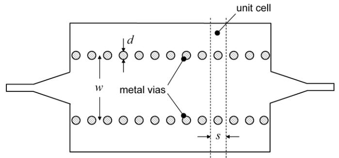
Figure 1. Geometry of SIW interconnect on paper.
