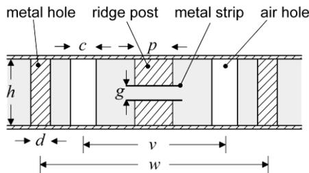
Figure 8. Geometry of the ridge substrate integrated slab waveguide ( $w=18.4$  mm,  $v=9.7$  mm,  $d=0.8$  mm,  $c=p=2.4$  mm,  $h=1.15$  mm,  $g=0.23$  mm).
