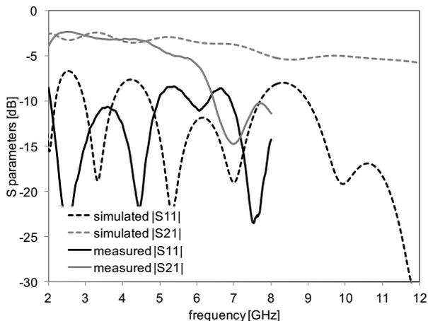
Figure 10. Simulated and measured scattering parameters of the ridge substrate integrated slab waveguide.
