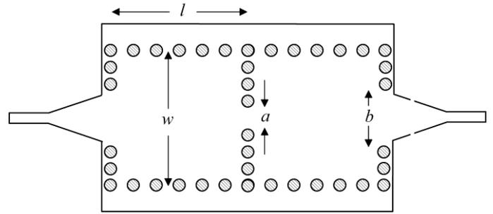
Figure 5. Geometry of the SIW filter on paper ( $w=24$  mm,  $a=14.27$  mm,  $b=15.89$  mm,  $l=19.17$  mm).
