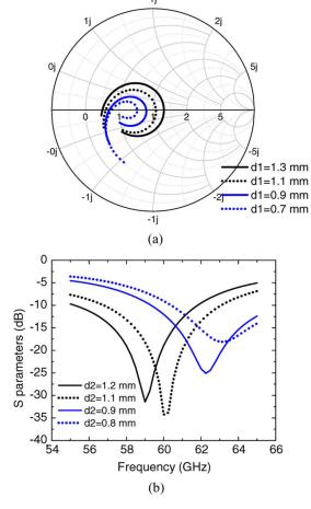
Fig. 4. (a) Input matching contours while varying  $d_1$ . (b) Reflection coefficient while varying  $d_2$ .
