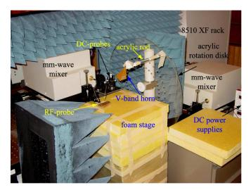
Fig. 11. On-wafer pattern measurement setup.
