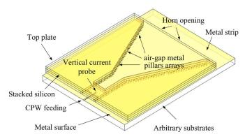
Fig. 1. 3-D view of the proposed micromachined horn.
