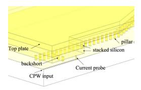
Fig. 2. The close-up schematic for the feeding structure (splitted along the symmetry plane).
