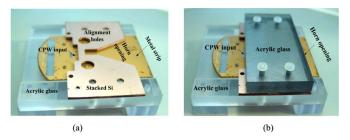
Fig. 10. Pictures of the horn antenna assembly.
