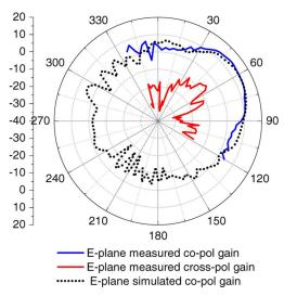
Fig. 12. Simulated and measured E-plane gain patterns.
