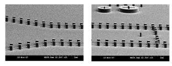
Fig. 8. SEM pictures for the micromachined horn showing the feeding probe and the horn flare pillar sidewall.
