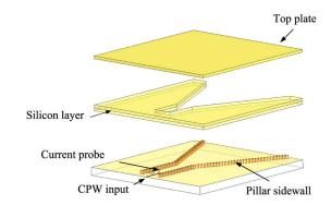
Fig. 9. The assembly scheme for the horn structure layer by layer.
