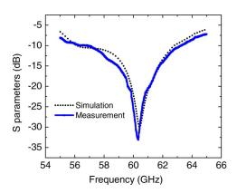
Fig. 5. Simulated and measured return loss of the proposed horn.
