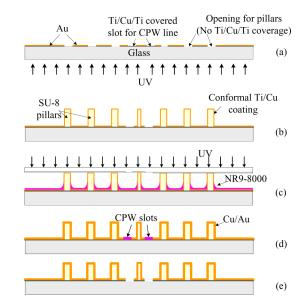
Fig. 7. Fabrication flow of polymer-core-condutor pillars.
