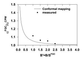
Figure 4: Attenuation of FGC waveguide with S=W=25  $\mu$ m normalized to the attenuation of conventional CPW with S=W=25  $\mu$ m as a function of the normalized ground plane width.
