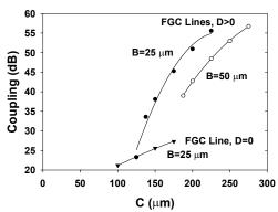
Figure 13: Coupling between FGC waveguides with D>0 and between FGC waveguides with a continuous ground plane (D=0) as a function of B and C determined by a 2D-FDTD analysis (S=W=25  $\mu$ m).
