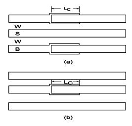
Figure 6: Schematic of MIM capacitor in the (a) ground planes and (b) center conductor of FGC waveguide.
