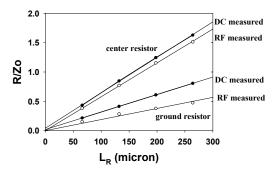
Figure 9: Measured resistance values of thin film resistor in FGC waveguide as a function of the resistor length.
