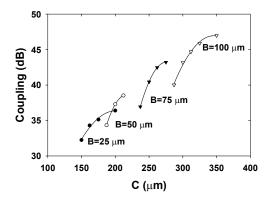
Figure 14: Measured coupling between FGC waveguides as a function of B and C (S=W=25  $\mu$ m).
