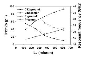
Figure 10: Measured series capacitance and self resonant frequency of MIM capacitors in FGC waveguide as a function of capacitor area.
