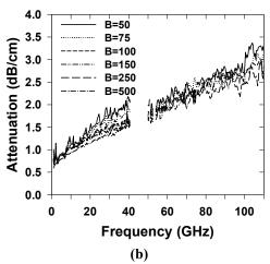
Figure 3: Measured attenuation of FGC waveguide as a function of frequency and ground plane width for (a)  $S=W=25 \mu m$  (b)  $S=W=50 \mu m$ .
