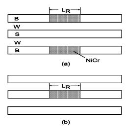
Figure 5: Schematic of thin film resistor in the (a) ground planes and (b) center conductor of FGC waveguide.
