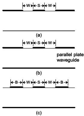
Figure 1: (a) Conventional coplanar waveguide (CPW), (b) Coplanar waveguide with lower ground plane, (c) Finite Ground Coplanar (FGC) waveguide.
