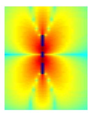
Figure 15: Horizontal electric field component of FGC waveguide (S=W=25  $\mu$ m, B=50  $\mu$ m).
