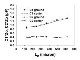
Figure 11: Measured shunt capacitance values of MIM capacitors in FGC waveguide as a function of the capacitor length.
