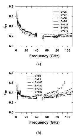
Figure 2: Measured effective dielectric constant of FGC waveguide as a function of frequency and ground plane width for (a) S=W=25  $\mu$ m and (b) S=W=50  $\mu$ m.
