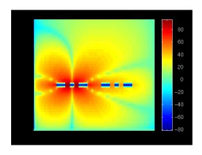
Figure 17: Horizontal electric field component of coupled FGC waveguides (S=W=25  $\mu$ m, B=50  $\mu$ m, D=75  $\mu$ m).
