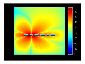
Figure 16: Horizontal electric field component of coupled FGC waveguides (S=W=25  $\mu$ m, B=50  $\mu$ m, D=25  $\mu$ m).
