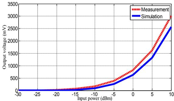
Fig. 6. The simulation and measurement results for the output voltage of the rectifier versus the input power.
