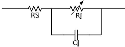
Fig. 3. The equivalent circuit of the schottky diode used in ADS.
