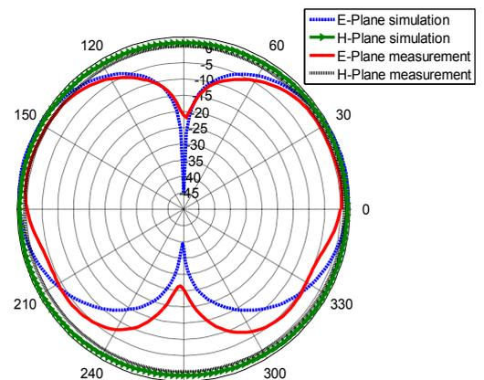
Fig. 9. The simulation and measurement results of the radiation patterns of the proposed antenna at 950 MHz.
