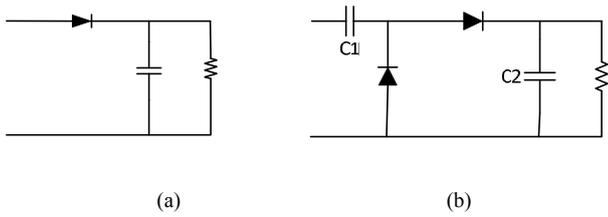
Fig. 2. (a) The schematic of the basic rectifier. (b) Voltage doubler.
