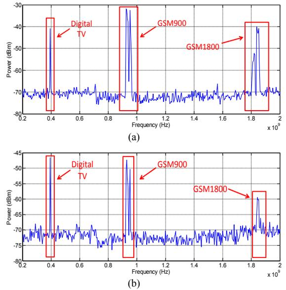
Fig. 4. The received power spectrum in (a) outdoor and (b) indoor environment.
