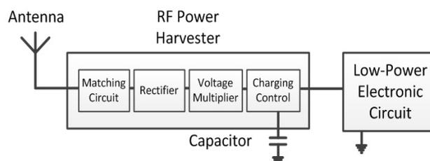
Fig. 1. The block diagram of a general power harvester.
