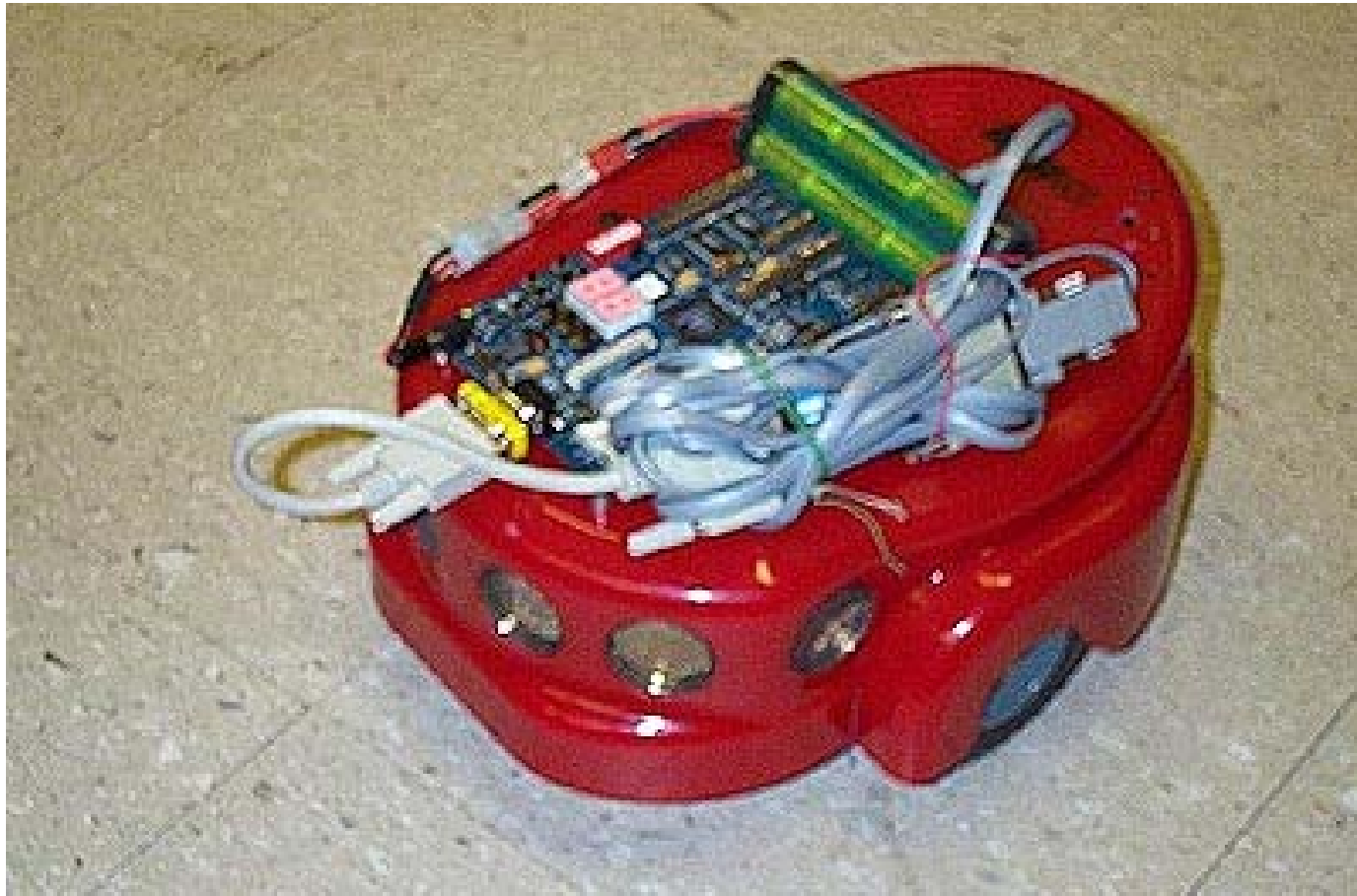
Figure 13.26 ActiveMedia's Amigobot robot base controlled by an FPGA with a Nios Processor
