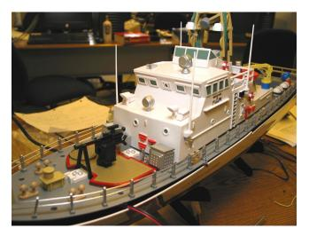
Fig. 4. This R/C toy boat was modified to create a robot boat. PIC microcontrollers, a GPS unit, an electronic compass, a gameboy camera, and a wireless modem are housed inside the cabin. Batteries serve as ballast inside the hull.
