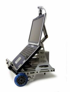
Fig. 8. The ER1 is a commercial robot base designed to carry a notebook PC.
