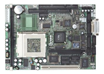
Fig. 10. This Arcom Olympus embedded computer board uses X86 PC chip technology and runs Windows CE or XP from Flash memory. Students are currently working on projects using it to control the Amigobot seen in Fig. 7.
