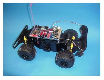
Fig. 3. This R/C toy truck was modified to create an autonomous robot by adding an FPGA board, IR sensors, and a compass. It has four-wheel drive and a suspension that is capable of moving on rough surfaces outdoors [3].
