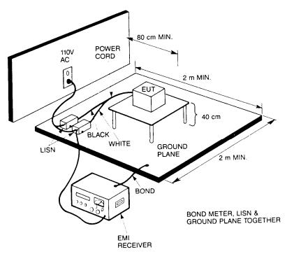
Figure 1-7. Test setup for FCC conducted emission measurements.
