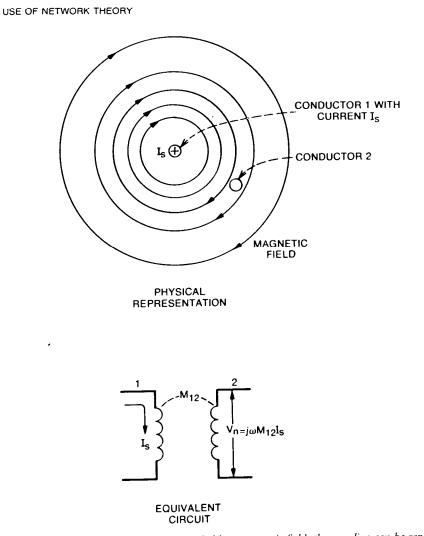
Figure 1-14. When two circuits are coupled by a magnetic field, the coupling can be represented as a mutual inductance.
