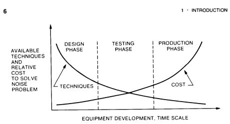
Figure 1-4. As equipment development proceeds, the number of available noise-reduction techniques goes down. At the same time the cost of noise reduction goes up.
