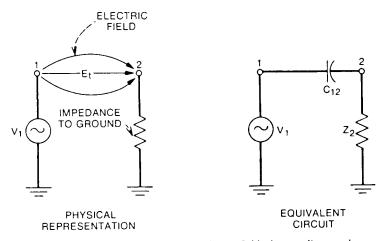
Figure 1-13. When two circuits are coupled by an electric field, the coupling can be represented by a capacitor.
