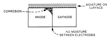
Figure 1-17. Galvanic action can occur if two dissimilar metals are joined and moisture is present on the surface.
