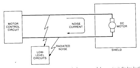
**Figure 1-12.** In this example the noise source is the motor, and the receptor is the low-level circuit. The coupling channel consists of conduction on the motor supply leads and radiation from the leads.
