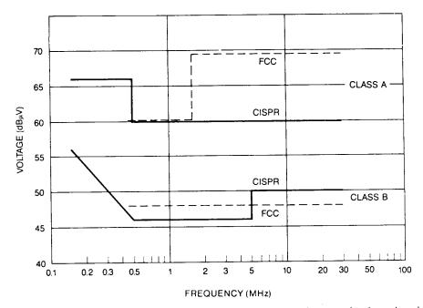
Figure 1-9. FCC Part 15. Subpart J and CISPR, Publication 22. narrowband conducted emission limits.
