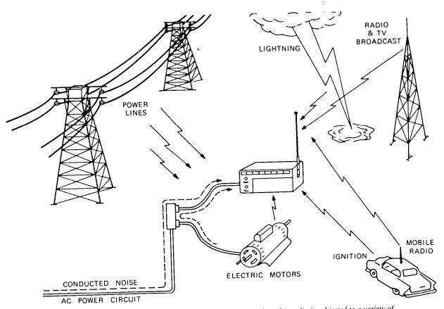
**Figure 1-2.** Outside of the laboratory, electronic equipment such as this radio is subjected to a variety of electromagnetic noise sources. Careful design is required to guarantee compatibility with the environment.
