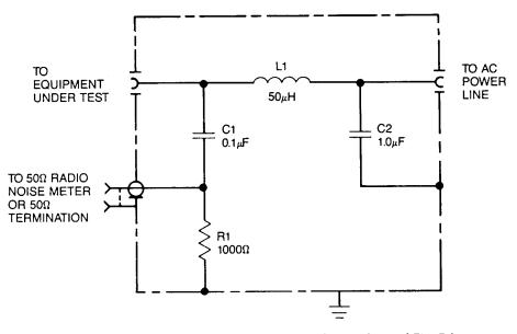
Figure F-4. Circuit diagram of LISN to provide the impedance of Fig. F-2.
