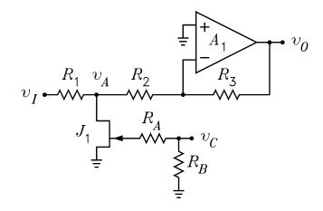
Figure 1: Basic VCA circuit.
