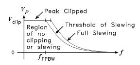
Figure 7: Maximum sine wave output voltage as a function of frequency.
