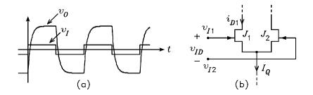
Figure 9: (a) Square wave input and output voltages. (b) JFET diff amp input stage.
