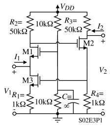
Use the Blackman's formula (see below) to calculate the smallsignal output resistance of the stacked MOSFET configuration having identical drain-source drops for both transistors. Express your answer in terms of all the pertinent small-signal parameters and then simplify your answer if  $g_m > g_{ds} > (1/R)$ . Assume the MOSFETs are identical.
