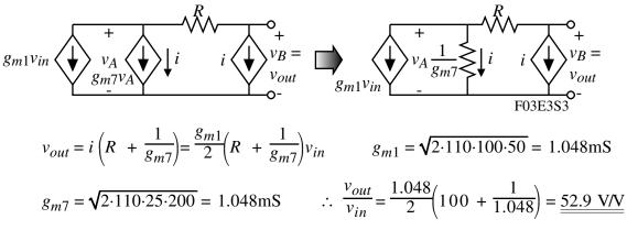
The approach to the second part of the problem will be to find the poles at A and B. The resistance to ground at node A is effectively  $R_A \approx 1/g_{m7} = 1/1.048$ mS and at node B to ground is  $R_B = R = 100$ k $\Omega$ . However, because of the shunt feedback at node B (and A) with a loop gain of 1, the output resistance is really 50k $\Omega$ . Therefore,
