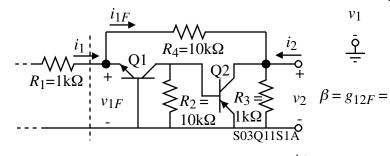
The open-loop ( $\beta = 0$ ) simplified ac schematic is given as,
