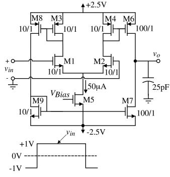
Similarly, when  $v_{in} = +1$ V,  $v_o$  is at -2.5V. When  $v_{in}$  switches back to -1V, all of the 50µA of M5 flows through M2 giving  $i_6 = 500$ µA and  $i_7 = 0$ . The rising propagation delay time is
