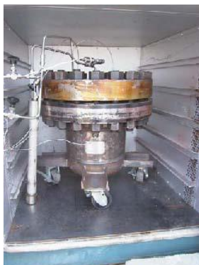
Figure 2: Ultra-high pressure vessel capable of maintaining a 100 Bar pressure Jovian environment, contained within the temperature vessel (oven). The microwave resonator is contained within the pressure vessel. The water reservoir is the large metallic tube at left.
