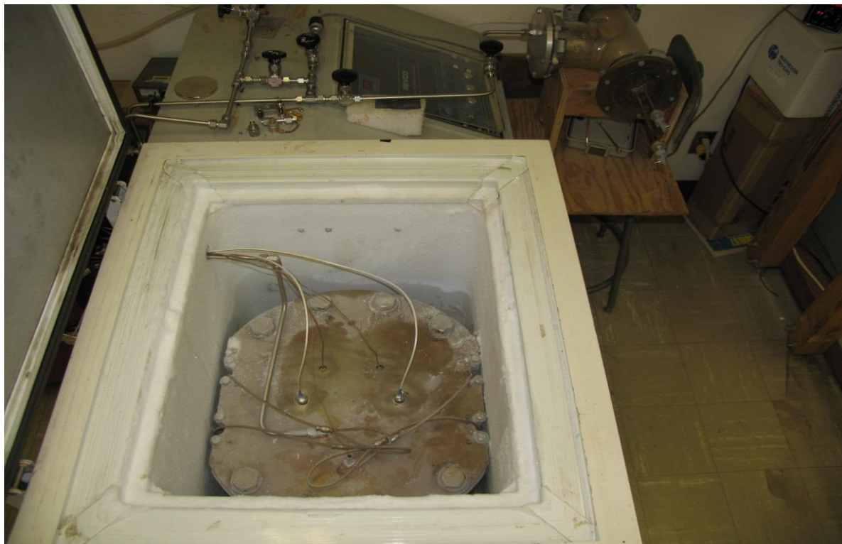
Figure 6: Medium-pressure vessel containing dual resonators placed in ultra-cold temperature chamber operating at 185 K.
