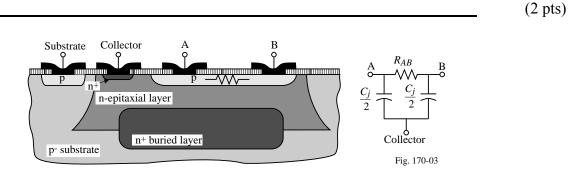
4.) If the collector-base junction was used as a junction capacitor, would adding the n+ buried layer
