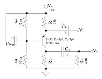
(b) Now replace the PNP with its small-signal model –use only variables,  $g_m$ ,  $r_o$ ,  $r_\pi$ ,  $C_\mu$ ,  $C_\pi$ , etc., where appropriate and applicable –do <u>*NOT*</u> use or calculate their respective absolute values–)–. (5 pts)
