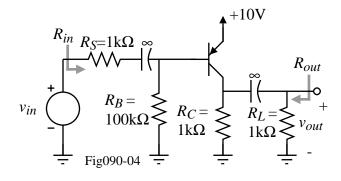
(b) Now draw the small-signal equivalent circuit (use variables only,  $g_m$ ,  $r_o$ ,  $r_\pi$ ,  $R_S$ ,  $R_B$ ,  $R_C$ , and  $R_L$  –do <u>NOT</u> use or calculate their respective absolute values–). (10 pts)
