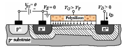
11. On the figure above, the effective threshold voltage <u>decreases / increases / remains constant</u> when the bulk-source voltage  $V_{BS}$  is increased from zero to 400 mV. (2 pts) 12. If a MOSFET's channel is only weakly inverted, its current is mainly due to <u>drift / diffusion /</u>
