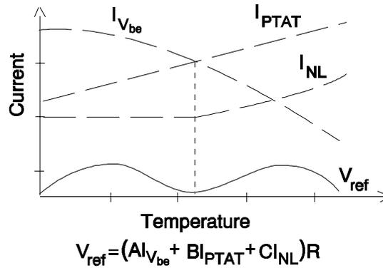
Figure 5.11. Temperature dependence of the curvature corrected bandgap.
