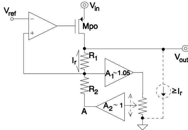
Figure 3.7. Widely adjustable low drop-out regulator structure.
