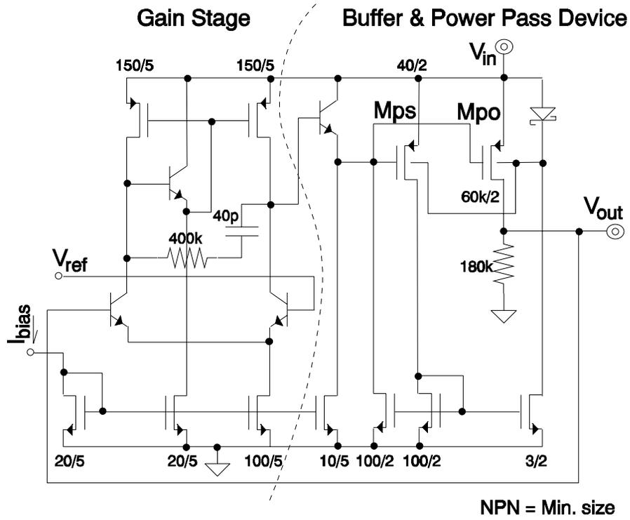
Figure 7.7. Schematic of the control loop circuit.
