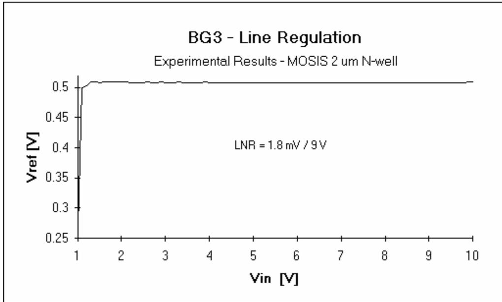
Figure 7.20. Line regulation performance of the reference.
