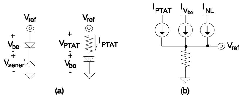
Figure 5.4. Output structures (a) voltage-mode and (b) current-mode.
