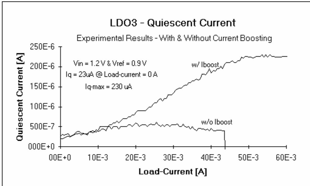
Figure 7.13. Quiescent current flow of the control loop.
