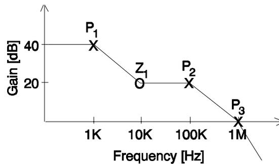
Figure 2.2. LDO frequency response under loading conditions.
