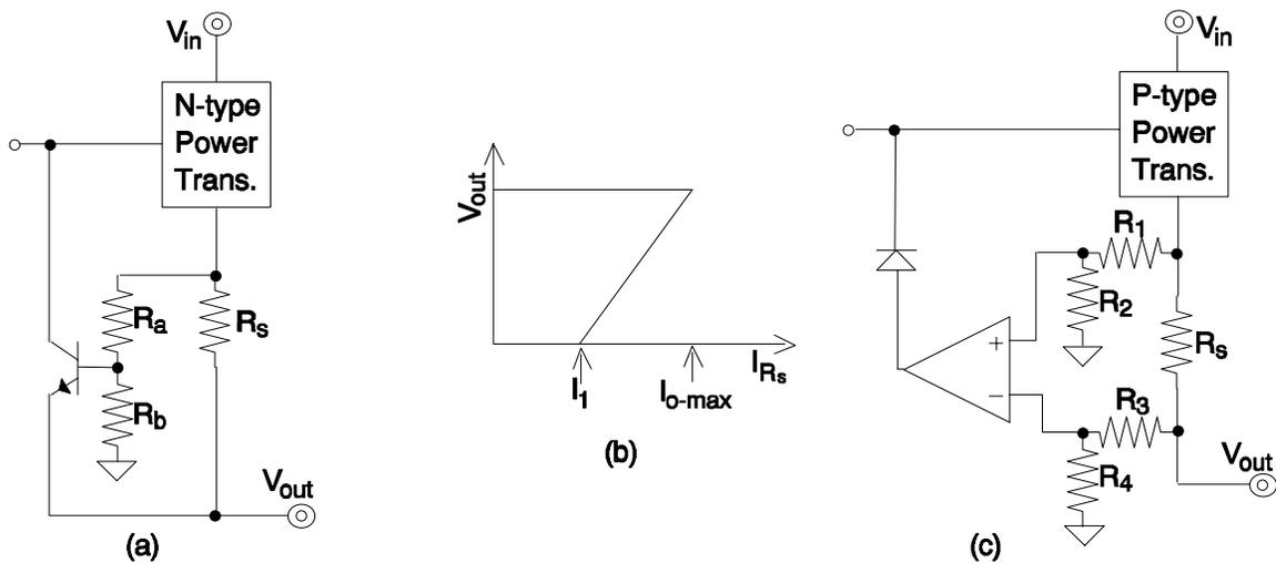
Figure 7.4. Foldback current limiting circuit protection.
