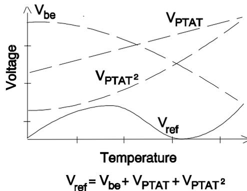
Figure 5.3. Squared PTAT curvature correction method for bandgaps.
