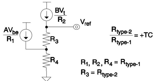
Figure 5.9. Temperature dependent resistor ratio curvature correction.
