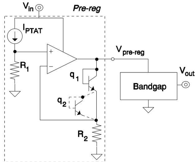
Figure 6.13. Pre-regulated supply voltage realization.
