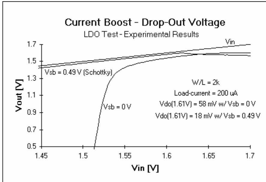
Figure 4.7. Drop-out voltage performance of the current boost topology.
