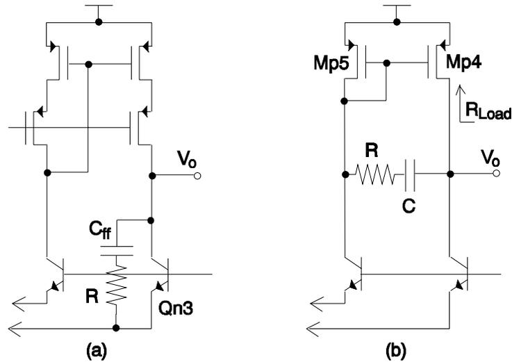
Figure 4.13. Variations of the frequency shaping amplifier.
