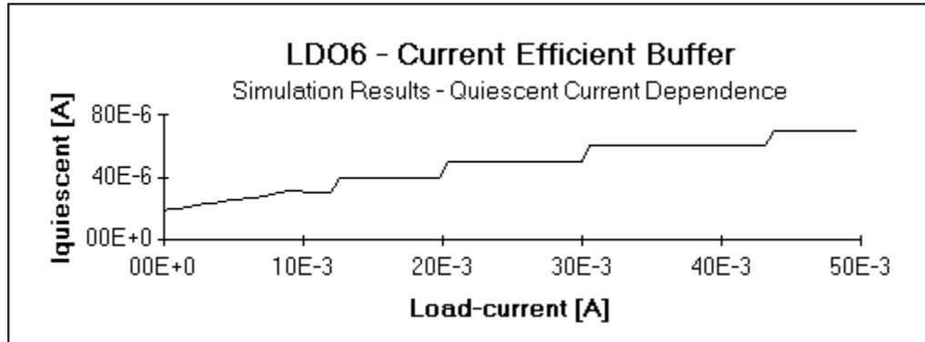
Figure 6.9. Quiescent current dependence of buffer on load-current.
