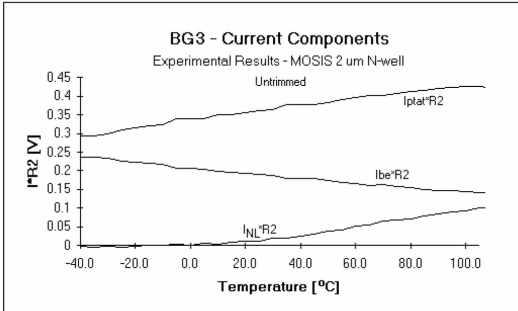
Figure 7.16. Temperature dependent currents in the reference.
