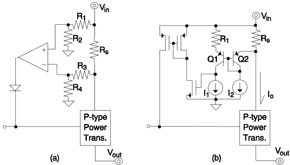
Figure 7.3. Low voltage current limiting circuit protection.
