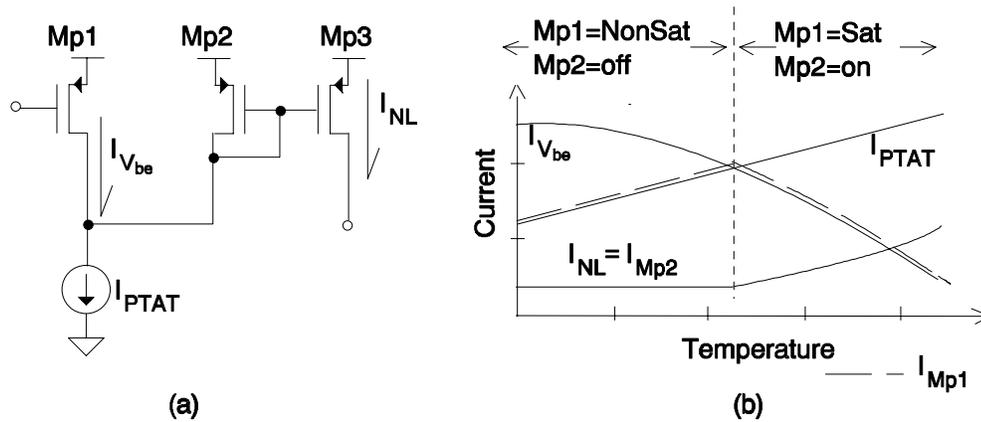
Figure 5.10. Current subtraction method for generating  $I_{NL}$ .
