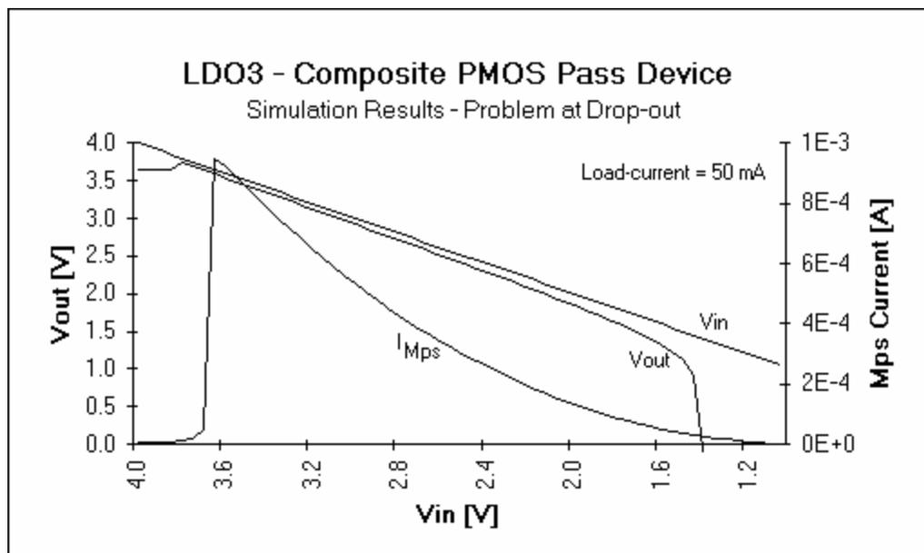
Figure 6.4. Simulation of current sensing problem at drop-out.
