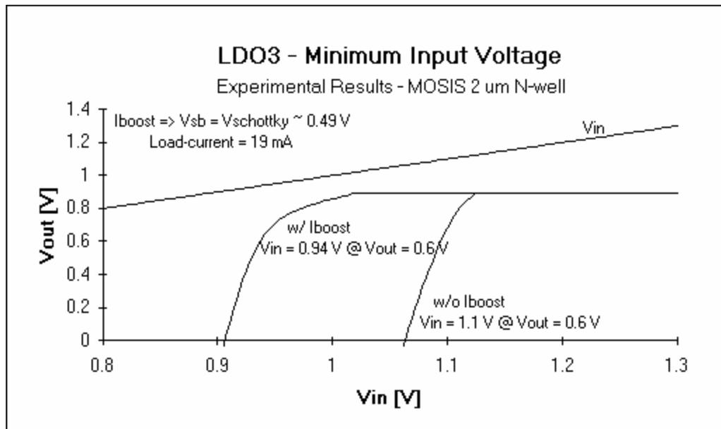
Figure 7.10. Minimum input voltage of the control loop.
