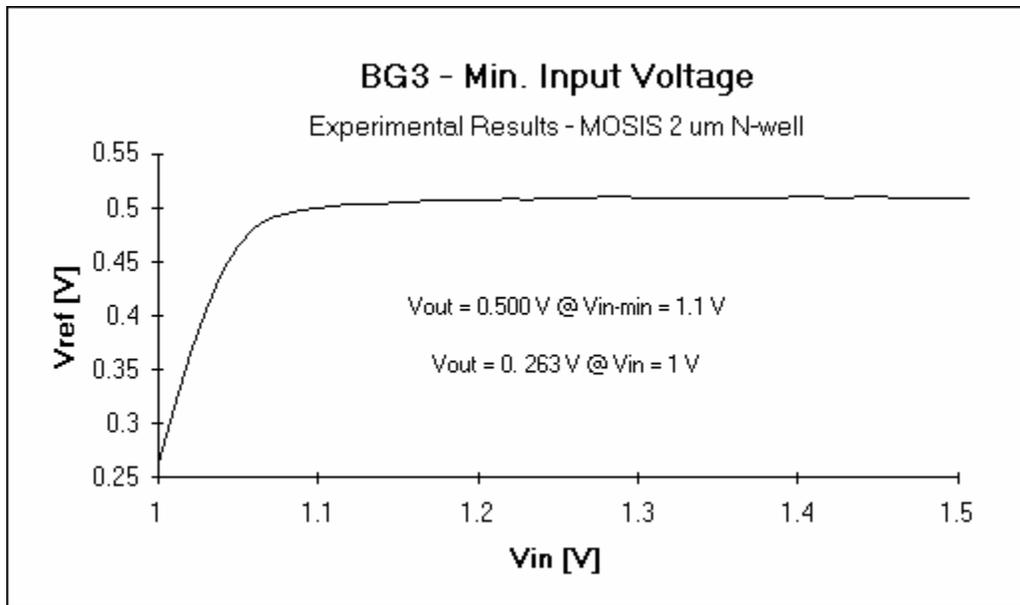
Figure 7.21. Minimum input voltage of the reference.
