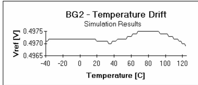
Figure 6.12. Temperature drift performance of the bandgap reference.
