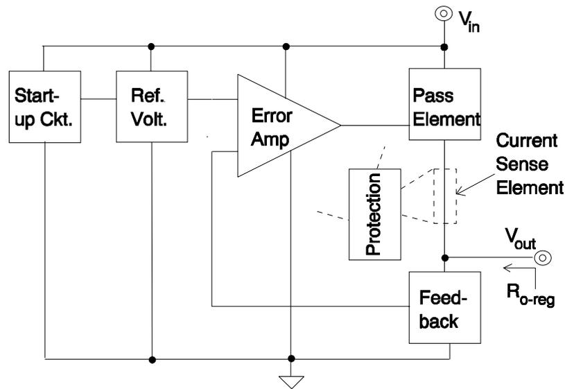
Figure 1.1. Generic low drop-out series linear regulator architecture.
