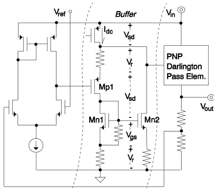
Figure 3.2. Buffered low drop-out regulator architecture.
