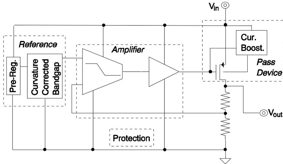
Figure 6.1. Block level diagram of the system.
