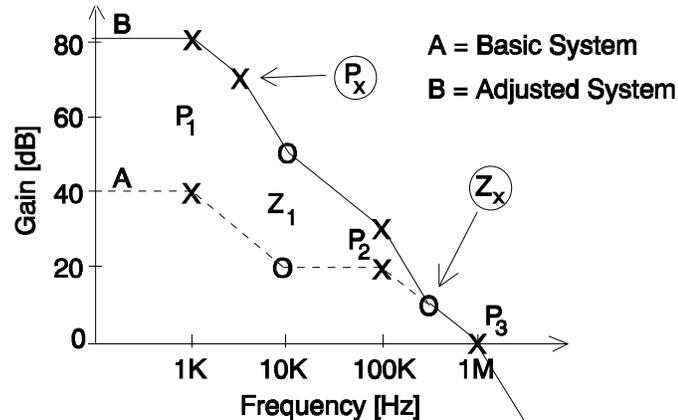
Figure 4.9. System's frequency response with an additional pole/zero pair.
