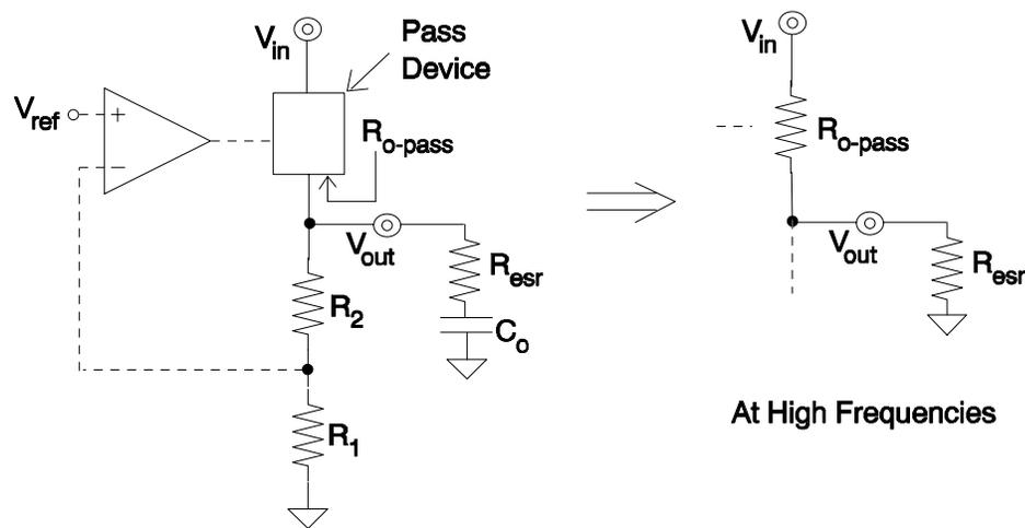
Figure 1.2. PSRR performance implications of high frequency operation.
