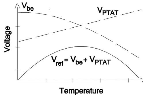
Figure 5.2. Temperature behavior of first order bandgaps.
