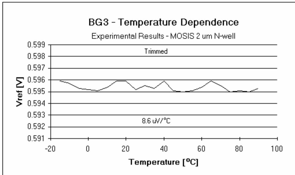
Figure 7.18. Temperature drift performance of the trimmed reference.
