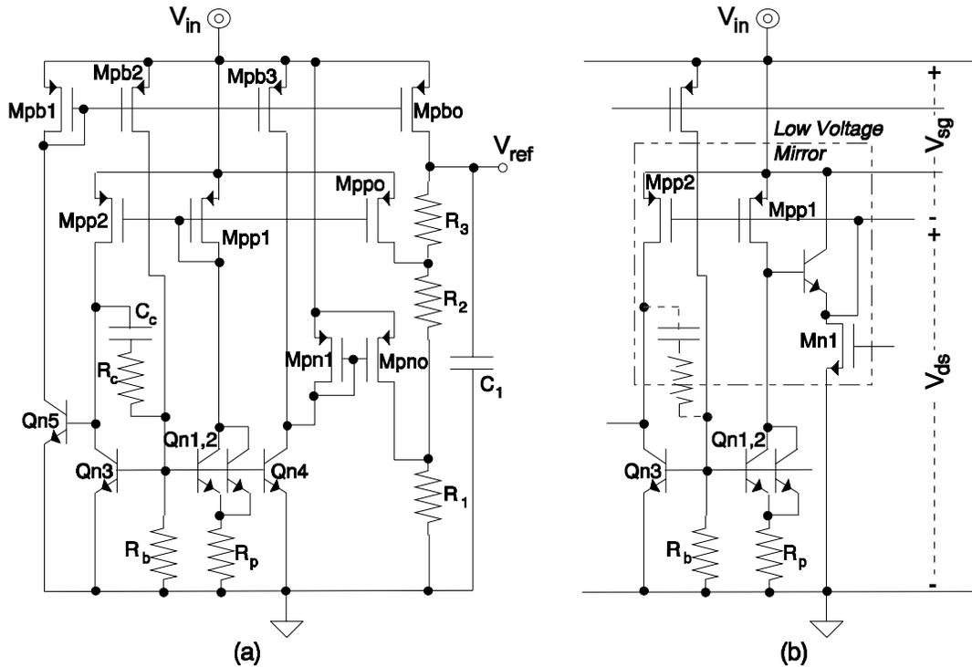
Figure 6.11. Bandgap with current subtraction curvature correction.
