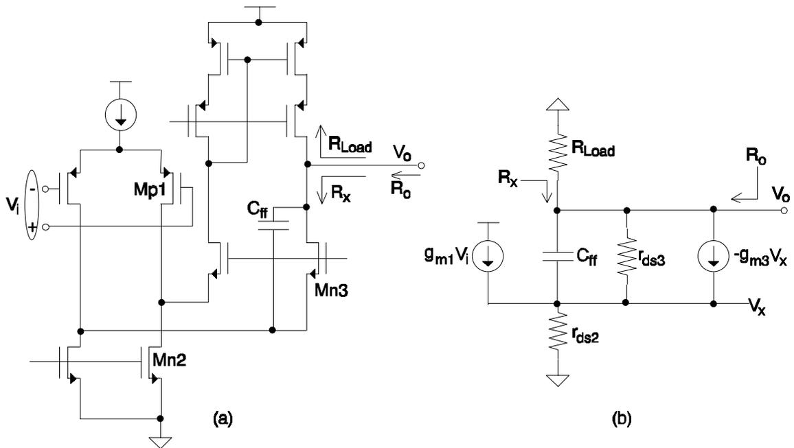
Figure 4.12. Pole/zero pair generation by a feed-forward capacitor.
