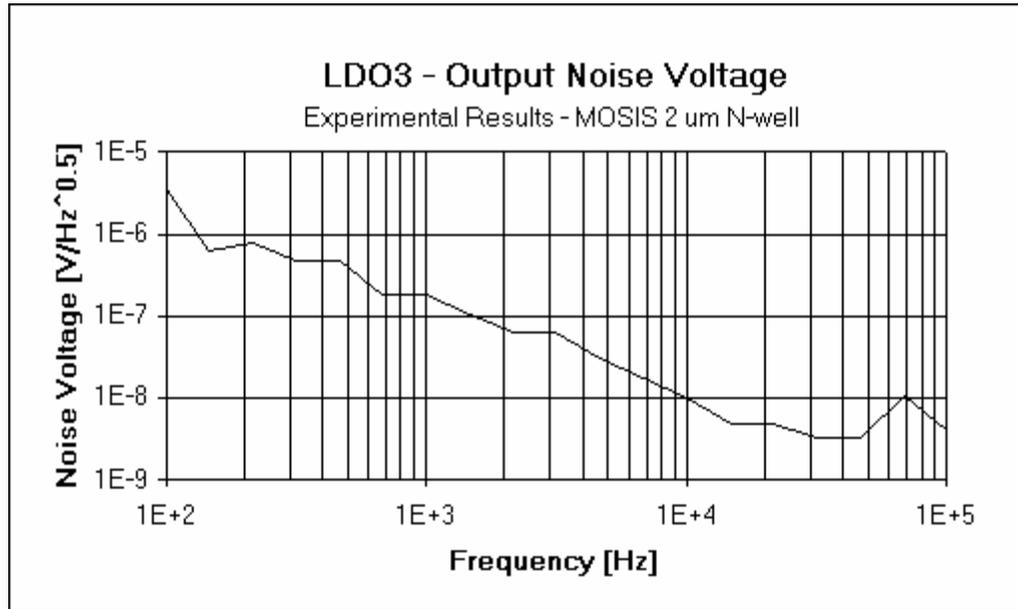
Figure 7.15. Control loop output noise voltage performance.
