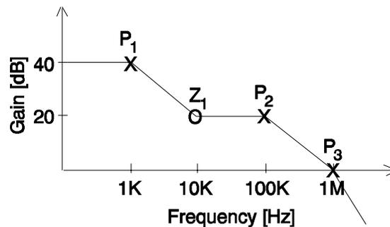
Figure 4.8. Linear regulator frequency response.
