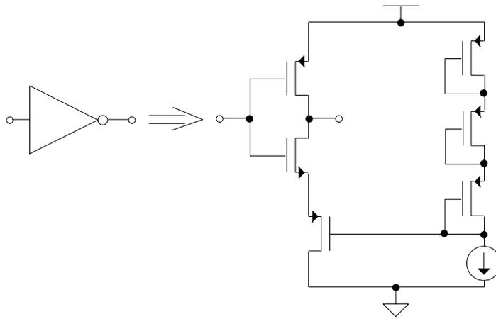
Figure 3.5. Digital inverter for the mixed-mode regulator.
