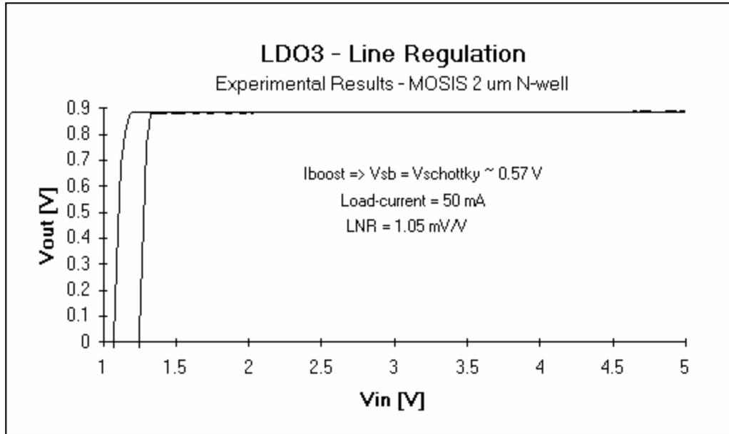
Figure 7.9. Line regulation performance of the control loop.
