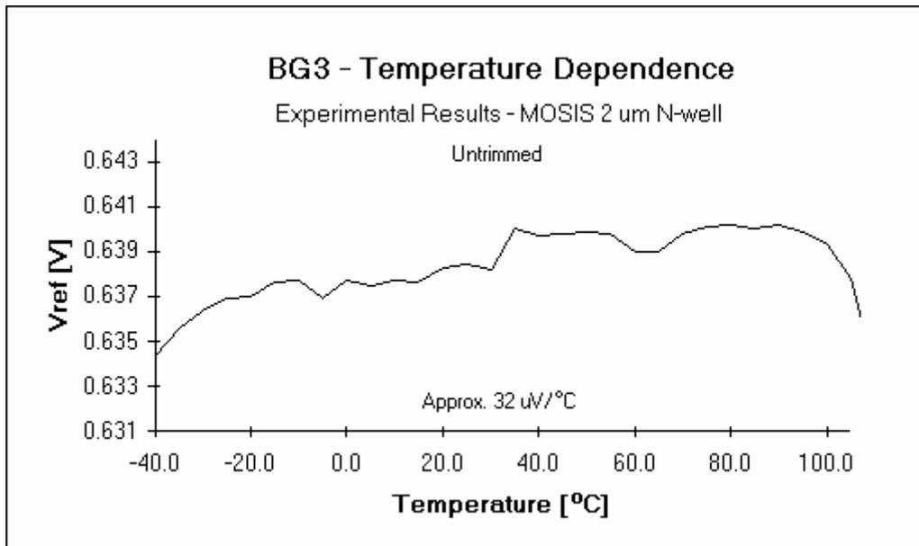
Figure 7.17. Temperature drift performance of the untrimmed reference.
