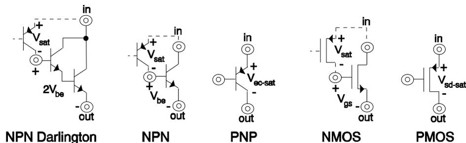
Figure 6.2. Pass element structures.
