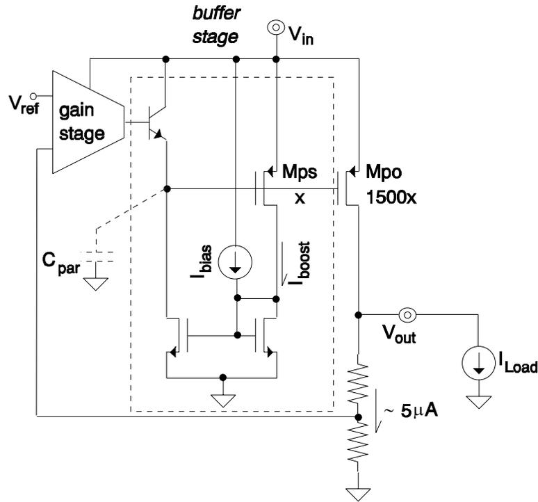
Figure 4.2. Current efficient-transient boost LDO buffer stage.
