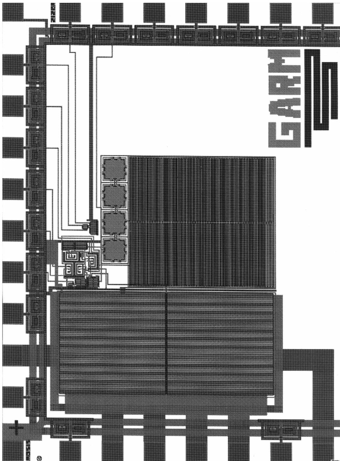
Figure C.3. Layout of the control loop (1103 x 1250  $\mu\text{m}$ ).
