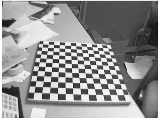
Fig. 3. One of twenty views of a checkerboard whose corners were treated as feature points to evaluate the DALT algorithm.
