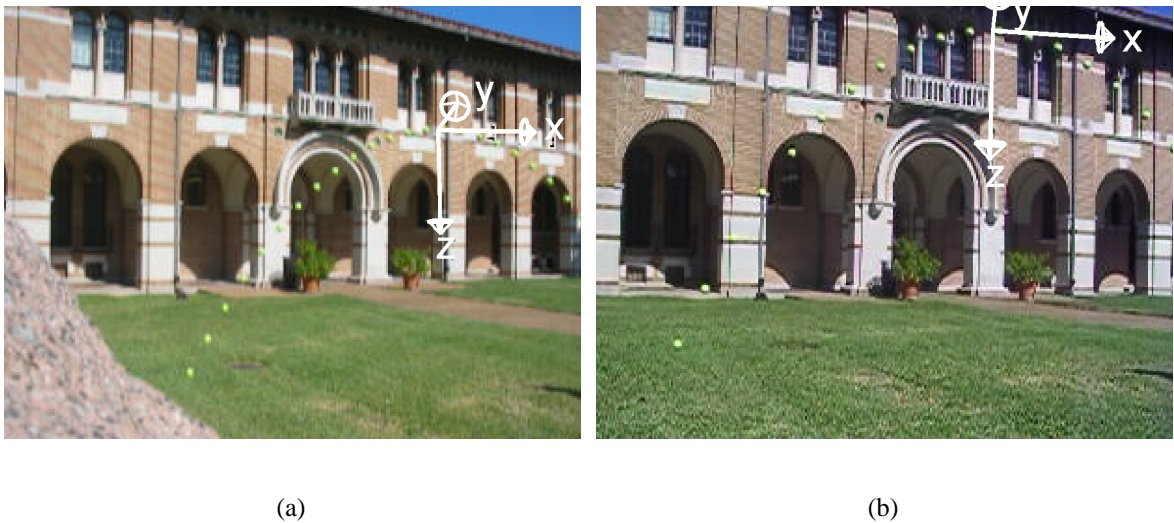
Figure 5.1 : Trajectory Estimation algorithm to localize several cameras by estimating local transforms between their own coordinate system and that of the trajectory. Shown in (a) and (b) are the mosaiced video streams from cameras a and b respectively with the estimated coordinate system \Gamma superimposed. Since Trajectory Estimation also solves the scale factor of similarity, we show one meter long arrows in 3-D space
