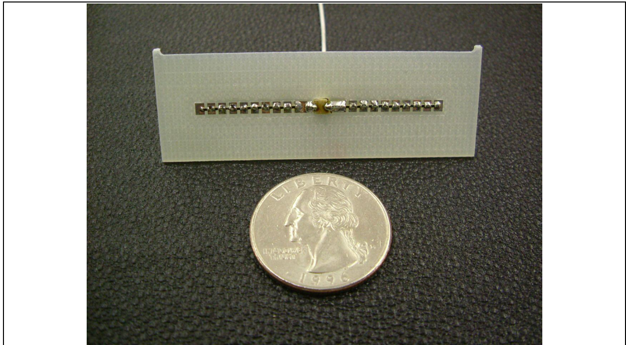
Figure 10. Resistively-loaded optical probe, 4 cm long.
