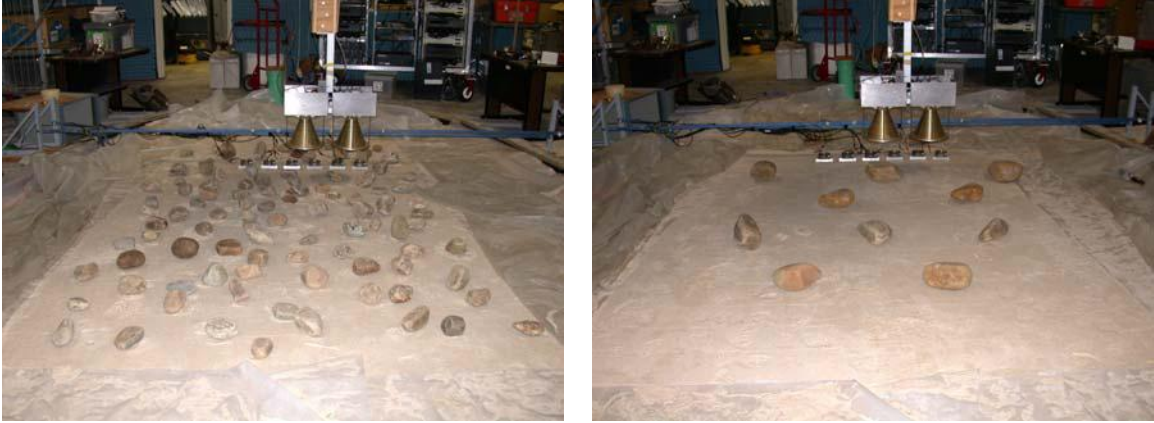
Fig. 14. The layout of the rocks before being buried below the surface. Rocks in the left image were buried first. The rocks in the right image were added subsequently.
