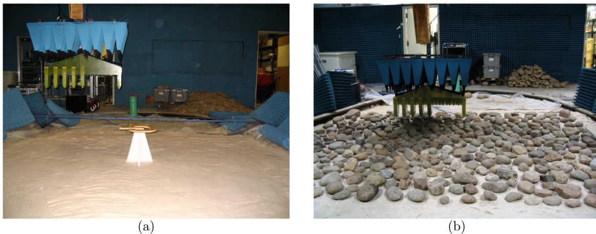
Figure 2. (a) Air target scan configuration, (b) Surface cluttered with river rocks.
