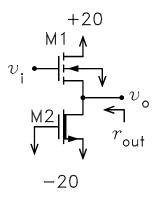
5. For the MOSFET, it is given that  $K = 0.001 \text{ A/V}^2$  and  $V_{TO} = 1.5 \text{ V}$ . Solve for  $I_D$ .
