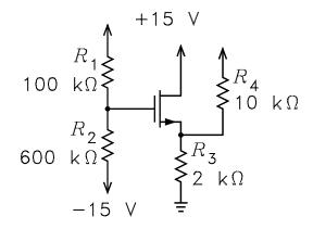
6. It is given that  $I_D = 2$  mA, K = 0.00075,  $V_{TO} = 2$  V,  $V_{DS} = 10$  V,  $\lambda = 0.02$ ,  $\chi = 0.4$ , and  $R_D = 10$  k $\Omega$ . The  $r_0$  in the figure is shown as an external resistor here. Solve for  $v_o/v_i$ ,  $r_{out}$ , and the input resistance seen by  $v_i$ .
