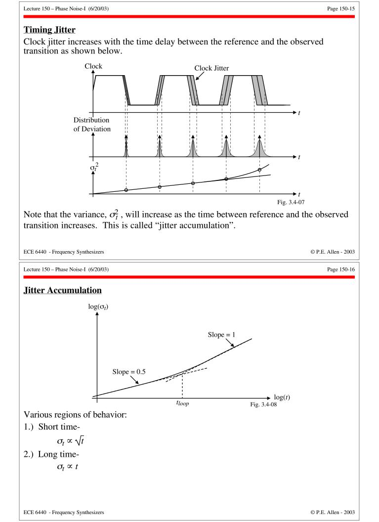
Start by observing that jitter is the standard deviation of the timing uncertainty,
