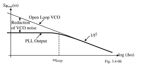
For offset frequencies below  $\omega_{loop}$ , the PLL can react to the noise variation of the VCO and compensate for slow random variations less than  $\omega_{loop}$ . For offset frequencies above  $\omega_{loop}$ , the PLL is unable to react fast enough to fast random changes in the VCO output and they appear directly on the output.
