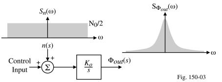
where n(s) is a white noise source with the double sideband power spectral density of  $N_0/2$ .
