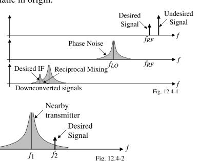
An oscillator's short term instabilities can be characterized in the frequency domain in terms of the single sideband noise spectral density.
