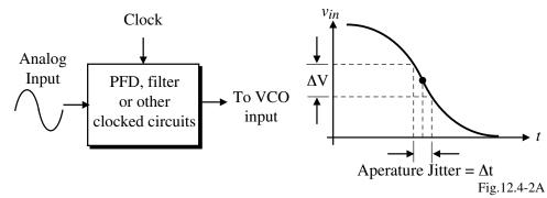
If we assume that  $v_{in}(t) = V_p sin\omega t$ , then the maximum slope is equal to  $\omega V_p$ . Therefore, the value of  $\Delta V$  is given as
