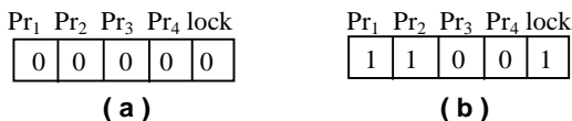
Figure 6. (a) Initial condition of lock and Pr bit locations in a four-processor system. (b) Bit values after PE3 acquired the lock, and PE1 and PE2 read the lock.
