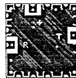
SUB pkg .375 x .375 x .11 (shown X2 actual size). Bottom View
