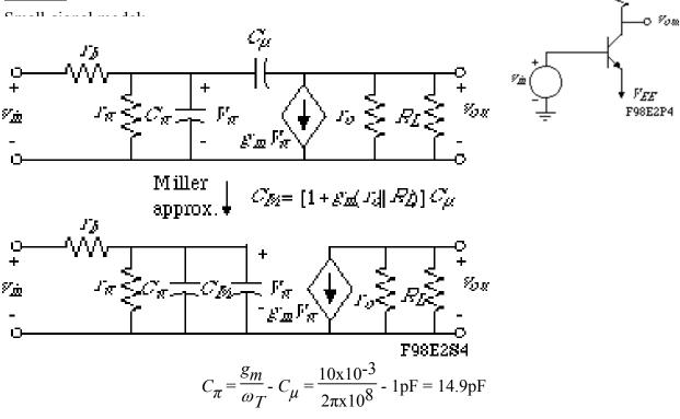
Method 1 –Miller Approx.:  $C_M = [1 + 10^{-2}(100k\Omega||10k\Omega)]1pF = (1+90.9)1pF = 91.9pf$ Thus,  $\omega_{-3dB} \approx \frac{1}{(r_b||r_\pi)(C_\pi + C_M)} = \frac{1}{99\Omega \cdot 106.8pF} = 94.6x10^6$  rads/sec.
